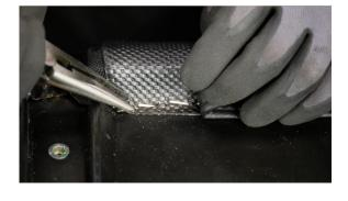
**NOTE:** It is not necessary to remove the entire seat cover. Be careful as to not rip the seat cover when taking out the staples and removing the back half of the seat cover.
